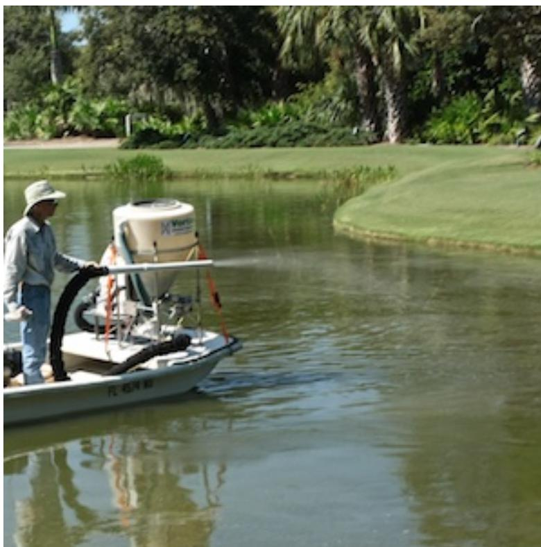
Figure 22. A Vortex™ TR-Aquatic for blowing pelleted formulations of fluridone (SonarONE®) at known rate; calibration is based on application swath width, vessel speed, and throughput of the blower assembly.
